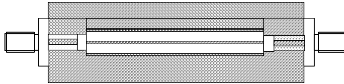
Figure 3d – Vertical cross section of test fixture with test set
